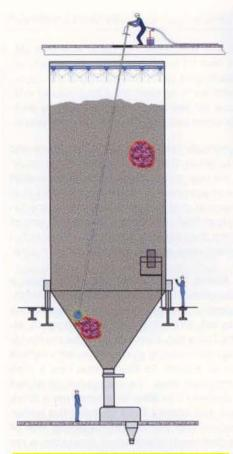
Fig. 1: Conduct a Thermal Scan to Assess the Hot Spot's size and location.
